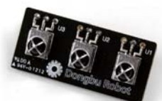
X1 DRI-0013 IR Receiver PCB
